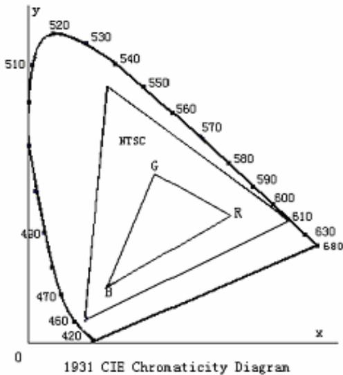
$$S = \frac{\text{area of RGB triangle}}{\text{area of NTSC triangle}} \times 100\%$$
