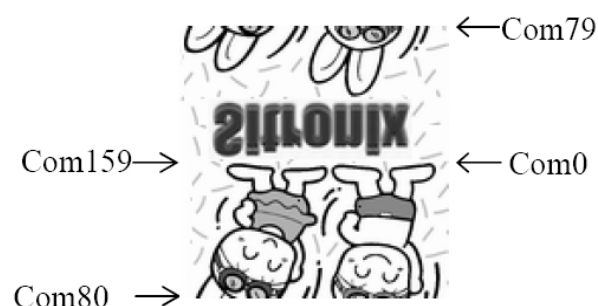
Figure 8.1.1 Common scan direction configuration
